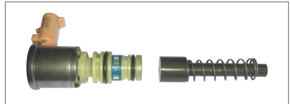
1996-Up On/Off Style 4L60-E. Sonnax spring works in this location.
