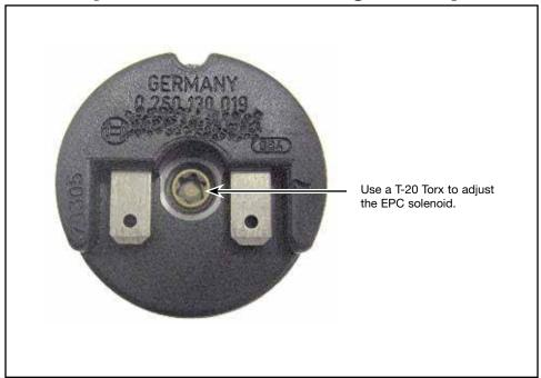
If this valve body is to be used in a Ranger pickup or Mazda B-series pickup with 2.3 or 2.5 L engine, the 1-2 shift and 3-2 coastdown shift may be too firm.
