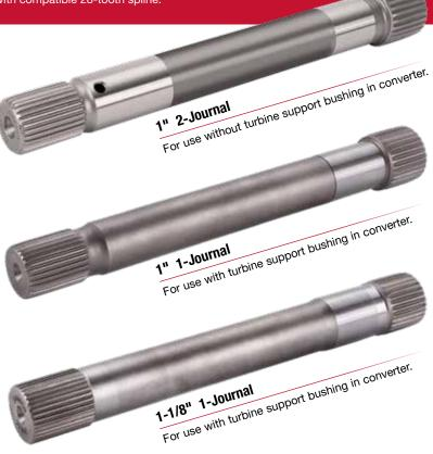
**Note:** Using this 1-1/8" shaft requires changing to a 35-spline turbine hub in the torque converter and use of Sonnax big shaft stator support tube kit 28154S-125 with larger inner diameter.
