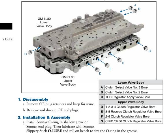
b. Carefully insert Sonnax O-ringed end plug into the bore just far enough to reinstall the OE retainer.
