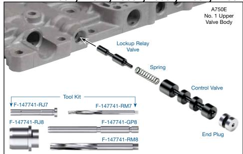
**IMPORTANT CAUTION:** Ream the small diameter inboard valve bore BEFORE reaming the larger diameter outboard bore. Failure to ream the smaller diameter inboard bore first will cause irreparable damage to valve body.
