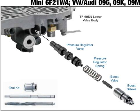
NOTE: Observe and record the step location of retainer on OE sleeve end prior to removal.
