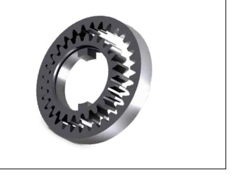
Sonnax oversized pump gears require machining to the gear pocket in the pump housing. It is important to maintain the OE center positions of the inner and outer gears in the pump housing. Sonnax pump gears are manufactured in sets, therefore, gear set components should not be separated or interchanged with other gear sets. Each individual pump gear set should be accurately measured and the pump pocket in the housing machined to fit within the clearances shown below.
