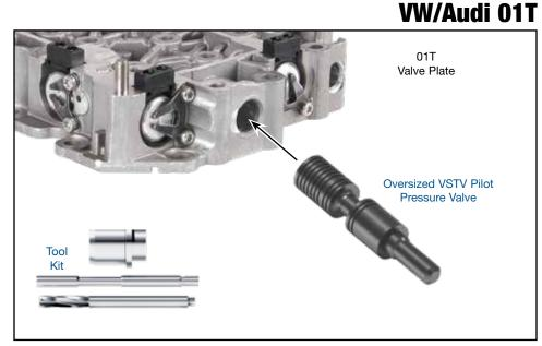
**NOTE:** Before beginning work, verify valve plate is 01T (**Figure 1**).
