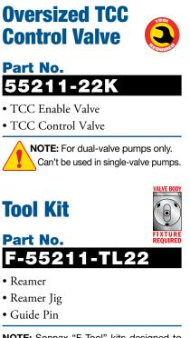
**NOTE:** Sonnax "F-Tool" kits designed to service a specific bore require the **VB-FIX**, a self-aligning valve body reaming fixture. For this valve kit, our specially designed oversized base plate **VB-06** must be also be used.
