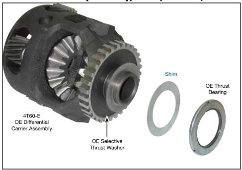
Sonnax shim **75410-10** installs between the differential carrier selective thrust washer and the bearing.
