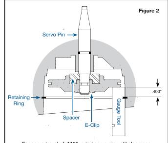
For servo travel of .115", grind servo pin until clearance between top of snap ring and bottom of piston equals .400".
