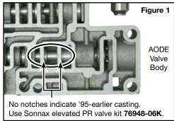
'96-Later Valve Body = Casting Notches Present
