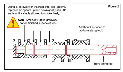
c. If Sonnax valve and/or sleeve do not move freely, reinstall bore sizing tool and tap tool back and forth using a hammer and screwdriver inserted through the ports and into tool grooves (**Figure 2**). Repeat process until valve strokes freely.
