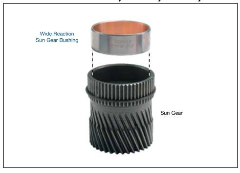
Install bushing using arbor press.
