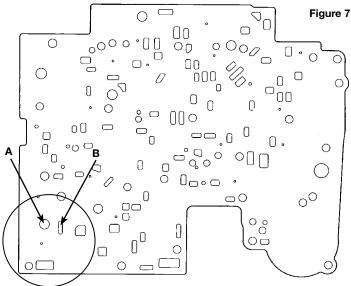
**NOTE:** Since the castings for PWM and non-PWM valve bodies are identical, this kit can be used when updating a non-PWM valve body for use in a PWM unit or retrofitting a PWM valve body for use in a non-PWM unit. The separator plate must also be changed when this is done (**Figure 7**).
