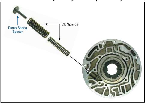
To install the Sonnax pump spring spacer, place the two OE springs over the spacer stem and reinsert into the pump cavity with the large spacer diameter seated against the pump wall. Refer to the picture above for proper arrangement.
