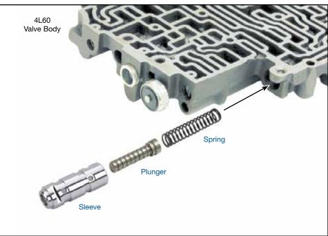
**NOTE:** Be sure to match OE plunger code (stamped on face of large plunger diameter) to Sonnax part number to ensure proper operation. Installing the wrong part can result in throttle pressure that is too high or low.
