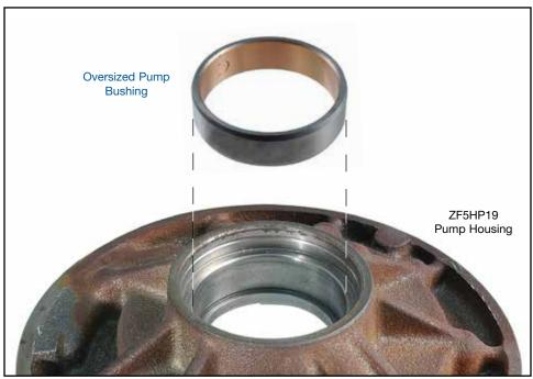
**NOTE:** This bushing is designed for damaged pump housings. The pump bore must be machined prior to installing Sonnax bushing. After bushing installation, bushing I.D. must be machined to set the desired clearance with the converter hub.
