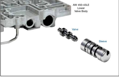
NOTE: The pressure regulator bore also is subject to extreme wear and should be vacuum tested at the port indicated (Figure 1). If the port fails to hold at least 14 in-Hg of vacuum, then the pressure regulator valve must be repaired to re-establish proper pressures.
