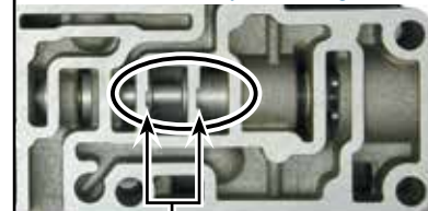
'96-Later Valve Body = Casting Notches Present
