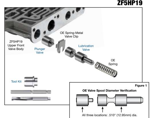
NOTE: The valve body section incorporating the lubrication valve bore also has three other valve bores. Removal of the end plate will release the valve trains in all four bores. Sonnax recommends removing all valve trains to thoroughly clean valve body after completing the lubrication bore reaming process. Do not mix up, discard or lose components from the valve trains. Return the valve train components from the other three bores to their original bores, in the order they were found.
