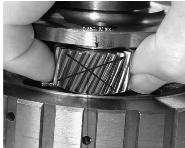
Inspect planet pins and endplay. No side to side movement
