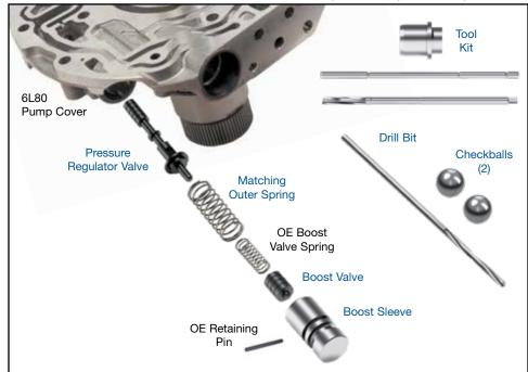
NOTE: In GM 6L45, 6L50, 6L80 and 6L90 units the pressure regulator valve and boost assembly are located in the pump cover. Transmission must be removed from the vehicle to access pump and replace the pressure regulator valve and boost assembly.
