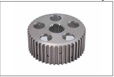
To ensure maximum clutch plate engagement with the hub splines, Sonnax 10-clutch hub **28304-01** is manufactured with a minimal chamfer at the indicated area.
