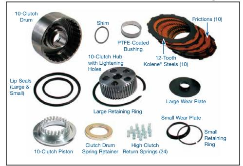
To ensure maximum clutch plate engagement with the hub splines, Sonnax 10-clutch hubs are manufactured with a minimal chamfer at the indicated area. When using non-Sonnax flanges, you must check the clearance between the chamfer on the hub and the sun gear flange to ensure there is adequate clearance. If more clearance is needed, machine a greater chamfer on the hub as necessary.
