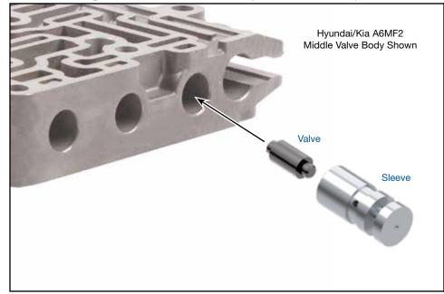
**NOTE:** Excessive wear can often be visually identified by shiny patches on inside diameter of sleeve. Wear can also be determined by vacuum testing, done through feed hole in OE sleeve. Using a small tip (available in Sonnax vacuum test stand kit **VACTEST-01K**) attached to the line, apply vacuum to one of the feed holes while covering hole on the opposite side. If sleeve fails to hold at least 18 in-Hg, install this kit.
