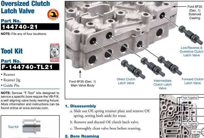
Ream clutch latch valve bore (for reaming instructions/ reamer care, please visit www.sonnax.com). Sonnax reaming tool kit F-144740-TL21 and VB-FIX are required for this operation.
