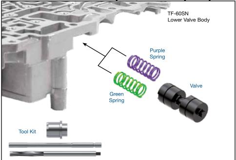
CAUTION: Prior to removal of spring adjustment plug, measure and record distance from plug to the casting (Figure 1). This dimension must be matched during reassembly.
