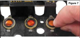
Place Sonnax laminate discs, then install D-rings flat side down.
