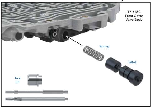
**CAUTION:** Prior to removal of spring adjustment plug, measure and record distance from end of plug to the casting (**Figure 1**). This dimension must be matched during reassembly.
