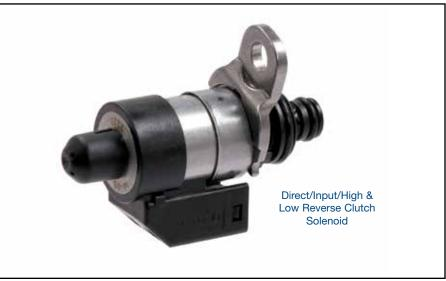
**NOTE:** Solenoids may be difficult to remove from valve body. Carefully twisting a flat-blade screwdriver between retainer bracket and valve body can ease solenoid removal. Alternately, a punch inserted from bottom of channel plate can be used to lightly tap solenoid snout outward.
