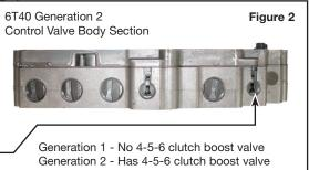
Also check the Transmission Control Module (TCM) identifications as shown in (**Figures 3** & **4**). The valve body and TCM must have the same Generation.
