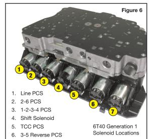
• Pressure Control Solenoid (PCS) 3-5 ohms at 70°F
