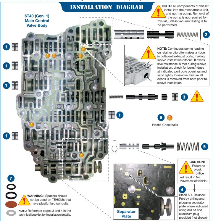
In addition to general rebuilding tips and technical information, the technical booklet included in this kit contains vacuum testing and additional repair options for higher mileage units or for repairing specific complaints which are beyond the scope of this kit.
