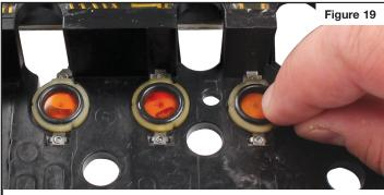
Place Sonnax laminate discs, then install D-rings flat side down.
