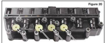
Plastic fluid conduits equipped on some solenoid bodies.
