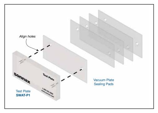
**NOTE:** Sonnax vacuum plate sealing pads are intended to be used on clean, dry surfaces. Oil and debris will degrade pad over time, causing discoloration, deformation and/or nicks and tears. The pad should be rinsed in water to remove surface dust and debris. If contamination eventually renders pad unusable, discard and replace with new pad.
