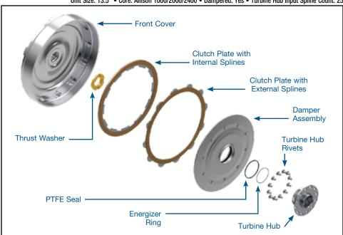
This performance converter kit combines the OE fluid coupling (impeller, stator and turbine) with all-new front cover, clutch plates, piston damper assembly and turbine hub to boost the converter capacity. The lockup clutch is not a salvaged OE clutch, it is a new and unique design.
