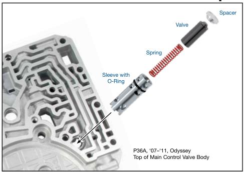
In addition to the application chart, the OE spring must match one of the following specifications:
