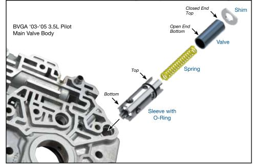
NOTE: Sonnax TC check valve kit is designed to fit in the main valve body, but will extend into the torque converter housing as well (Figure 1). Once main valve body and regulator valve body are assembled to the torque converter housing, the sleeve should occupy the entire height between those castings.
