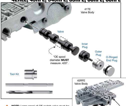
NOTE: Large spool of OE switch valve must be .420" dia. (main photo). If spool measures .420", continue installation. If spool measures .453", STOP! This Sonnax kit cannot be used.
