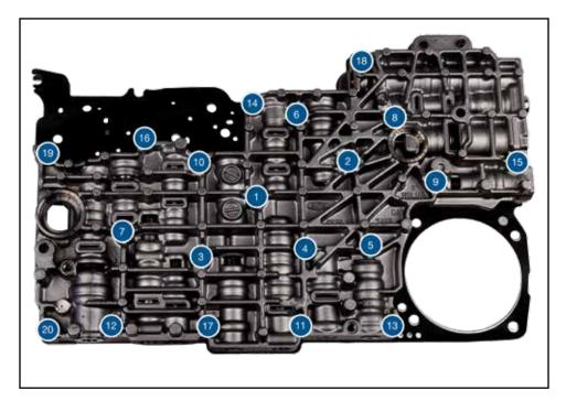
Torque valve body bolts in sequence shown: 89 in-lb
