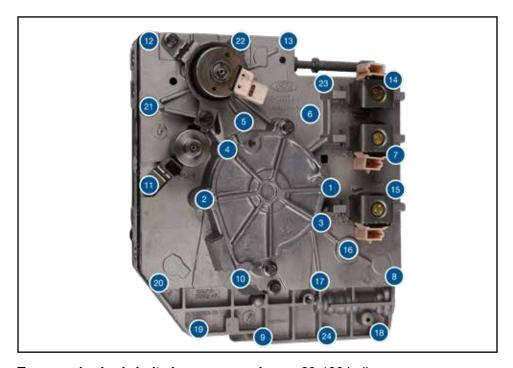
Torque valve body bolts in sequence shown: 80-106 in-lb
