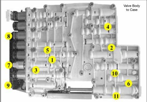
Torque valve body bolts in sequence shown: 53 in-lb
