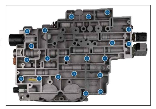
Torque valve body bolts in sequence shown: 97 in-lb
