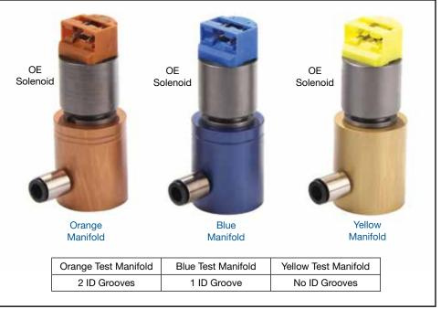
**NOTE:** Sonnax test manifold kit can prove or disprove internal mechanical sealing ability only; it does not test the integrity of the electrical coil and contacts. While internal mechanical sealing problems are the leading cause of failure for this family of solenoids, electrical testing should also be carried out to confirm comprehensive solenoid operation.
