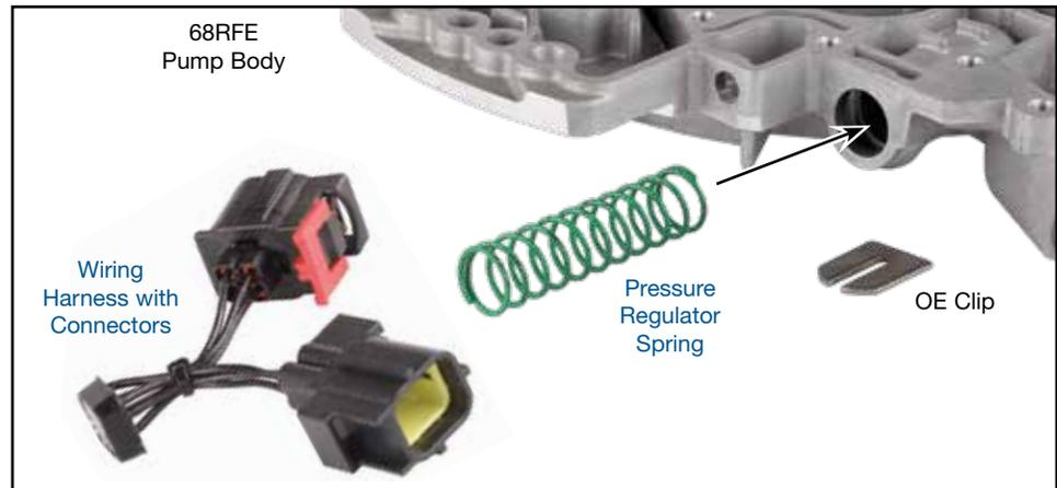
**NOTE:** This kit is not recommended for use with transmission tuning mods. If you are unsure of the vehicle's programming, use a scan tool to verify transmission line pressure meets stock levels (Drive at idle = 60 psi, Drive under heavy load = 160 psi). If desired line pressure values are greater than this, the system most likely has aftermarket tuning mods to the transmission pressure.
