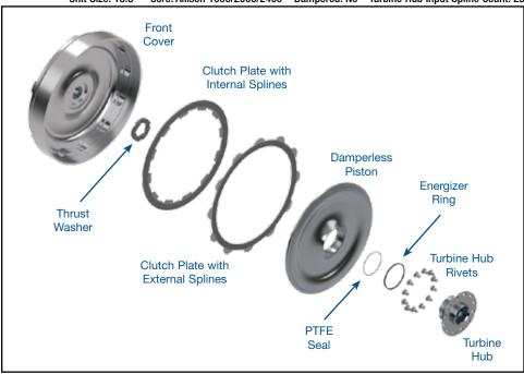
This performance converter kit combines the OE fluid coupling (impeller, stator and turbine) with all-new front cover, clutch plates, piston and turbine hub to boost the converter capacity. The lockup clutch is not a salvaged OE clutch, it is a new and unique design.
