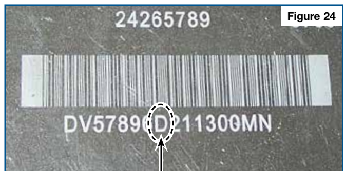
Figure 24 Generation 2 & 3 TCM Identification Number: Eighth digit under bar code is a Letter, starting with B, C or D.
