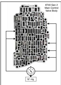
**NOTE:** Vacuum test end plugs at outboard port while sealing bore opening with thumb.
