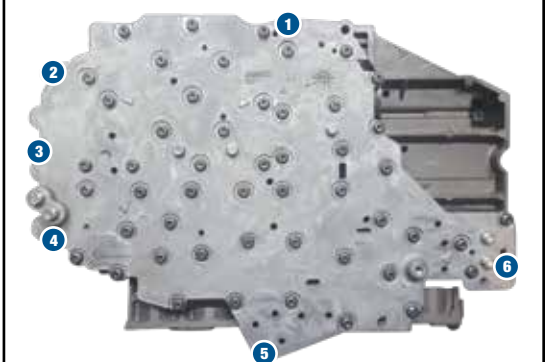
Install six (8mm) head bolts and torque to 105 in-lb. Figure 3
