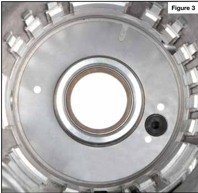
Sonnax grommet and shim installed in case ( Figure 3 ).
