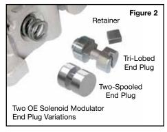
plug into orifice and peen shut.
