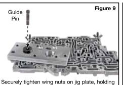
Securely tighten wing nuts on jig plate, holding all components together, while letting Sonnax guide pin move freely in OE accumulator bore.
