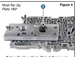
Setup: Position #3 Jig Plate & Reamer Jig
