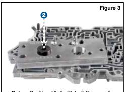
Setup: Position #2 Jig Plate & Reamer Jig
